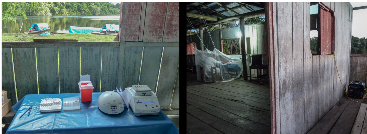
Fig 3. Laboratory set-up for 'POC-LAMP testing' in the community.
