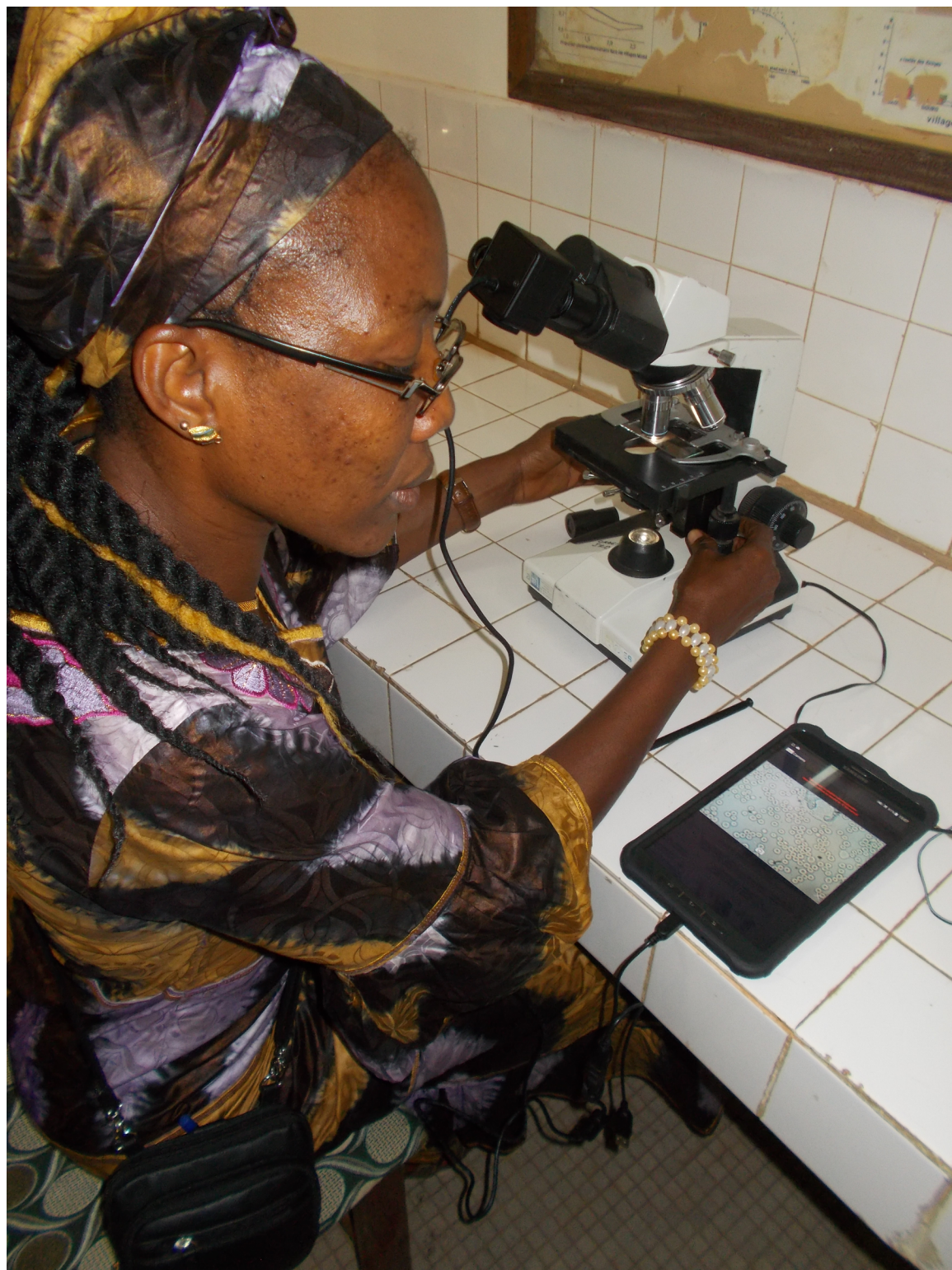
Fig 2. Digital imaging system for recording videos of microscopic images using an android tablet and external camera mounted onto the ocular tube of a microscope.
