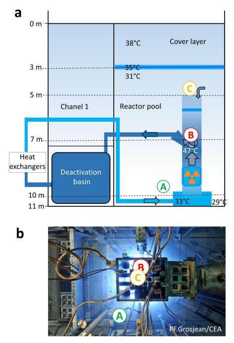
**Figure 1.** Configuration of the Osiris reactor's pool (adapted from [11]) and sampling points A (pool's bottom), B (inside the core unit), and C (above the core unit). (a) Schematic view, (b) top view. At shutdown, the radiation dose rate reached 25 Gy/h at point B, 15  $\mu$ Gy/h at point C, and was below 0.1  $\mu$ Gy/h at point A.
